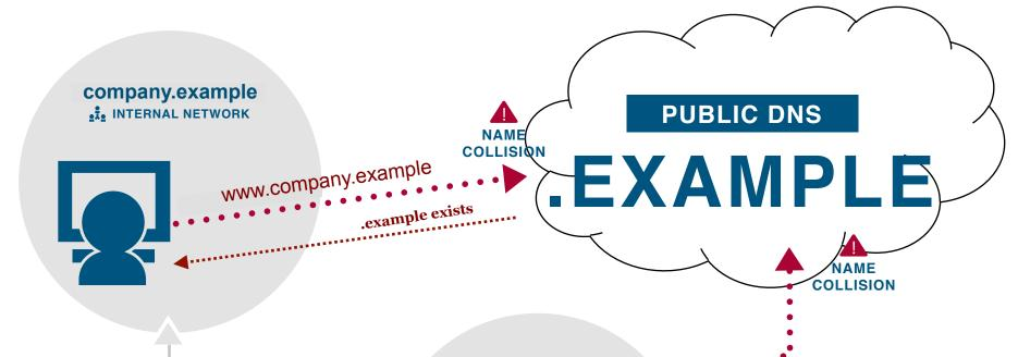
Private network configured in such a way that could "leak" the request to the public Domain Name System, when using a name in a private network matching a name in the public DNS
