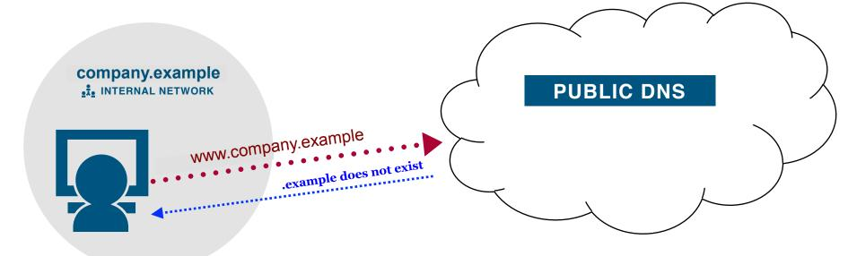
Private network configured in such a way that could "leak" the request to the public Domain Name System, when using a name in a private network that does not exist in the public DNS
