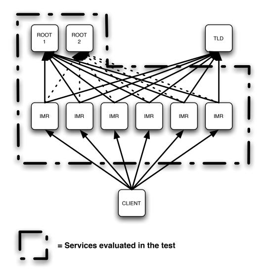
Figure 1: Service topology for the test
